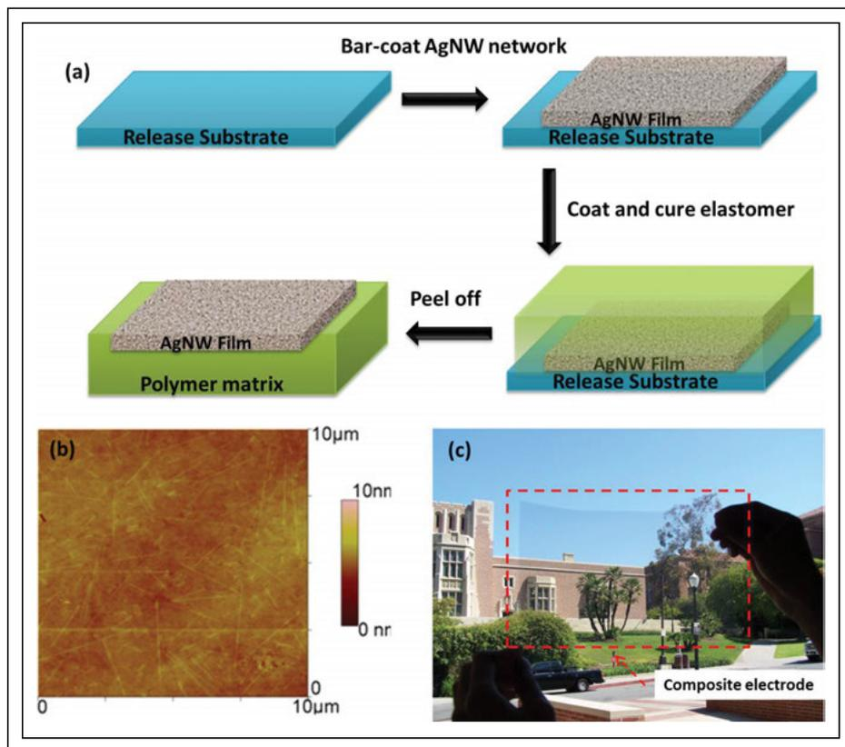
**Fig. 1:** At top (a) is a schematic illustration of the manufacturing process of an elastic transparent silver-nanowire-PUA composite electrode. An atomic force microscopy (AFM) topographic image of the silver-nanowire-PUA composite electrode appears in (b). And (c) is an optical image of a silver-nanowire-PUA composite electrode (25 cm × 15 cm, within the red dashed rectangle).
