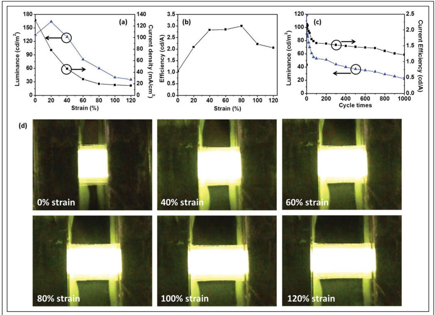
**Fig. 5:** The chart at upper left (a) depicts current-density and luminance characteristics of a PLEC device at 12 V with increasing strains. Chart (b) shows current-efficacy characteristics of the device with strain and chart (c) plots the luminous efficacy at 0% strain during 1000 continuous cycles of stretching–relaxing between 0 and 30% strains. In (d) are photographs of a PLEC (original emission area: 5.0 mm × 4.5 mm) biased at 14 V at specified strains.
