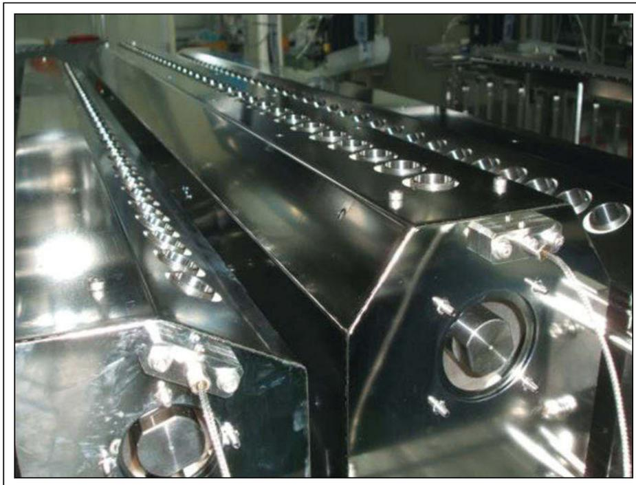
Fig. 2: This linear-nozzle-source deposition equipment is from Sunic Systems in Korea.
