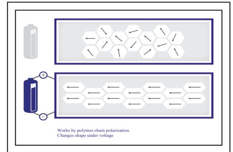
Fig. 4: This electro-mechanical polymer working mechanism shows the elongation of the materials in the lower box.
