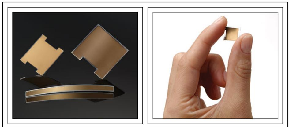
Fig. 2: Electro-mechanical polymers (EMPs) are a new type of device capable of providing haptic responses in a small form factor.
