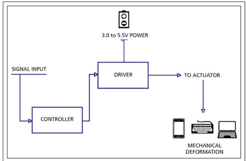
Fig. 6: A typical haptic system architecture consists of a microcontroller, driver and power electronics, and one or multiple actuators and sensors.
