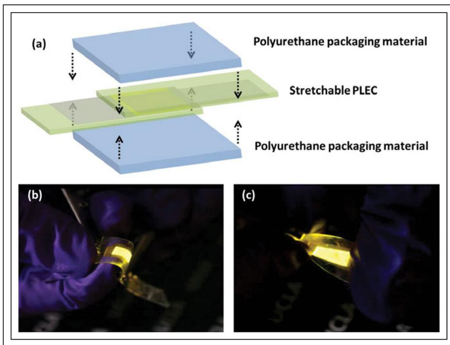
**Fig. 6:** At top (a) is a depiction of the lamination of an elastomeric PLEC device between two layers of a polyurethane packaging material. Below are images of an encapsulated PLEC device that is (b) stretched, bent, and wrapped around a finger and (c) formed into a twisted shape.
