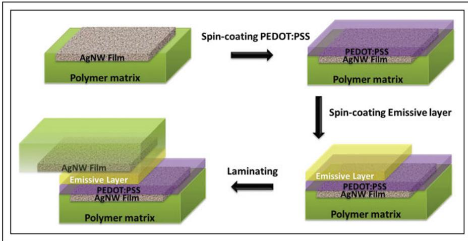
**Fig. 3:** This simplified rendering shows the fabricating process for a stretchable PLED device based on a pair of silver-nanowire–PUA composite electrodes (not to scale). The processes are all-solution based (AgNW = silver nanowire).
