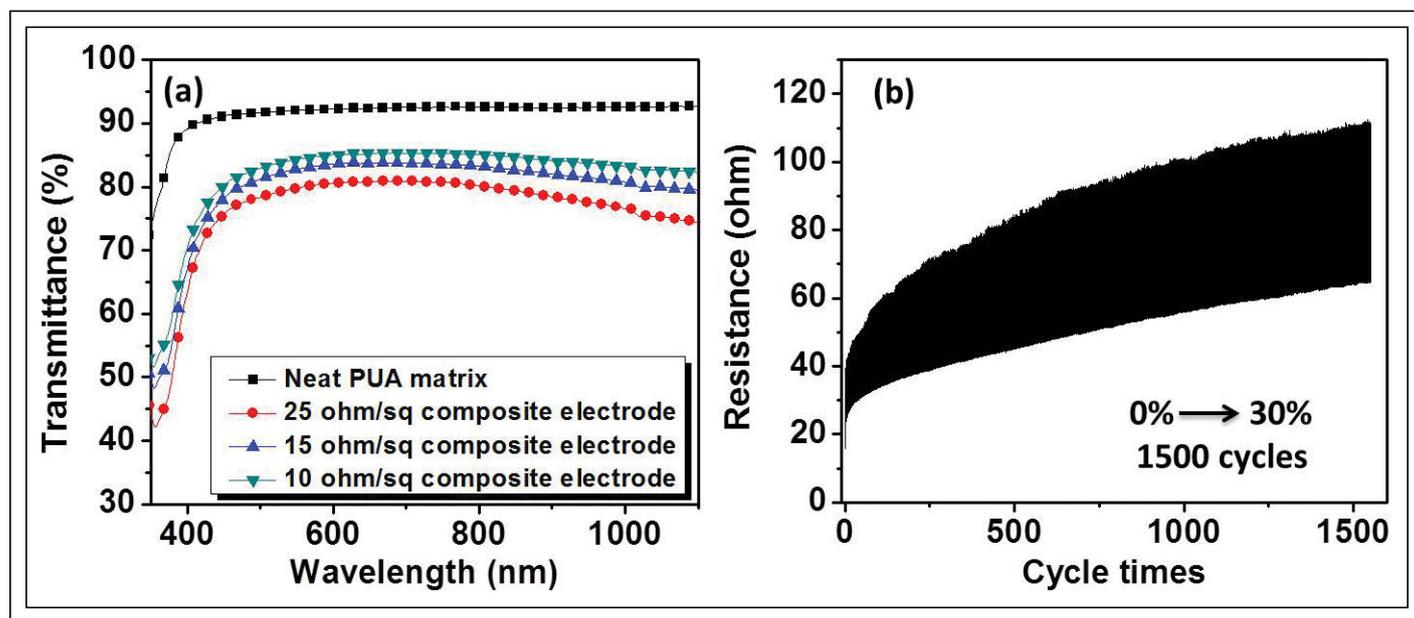
**Fig. 2:** At left (a) are the transmittance spectra of a neat PUA film and silver-nanowire-PUA composite films with a specified sheet resistance (thickness  $\sim 150 \mu\text{m}$ ). At right (b) is a graph representing transient resistance measured during 1500 cycles of stretching-relaxing between 0% and 30% strains for a  $15 \Omega/\text{sq}$  silver-nanowire-PUA composite electrode.
