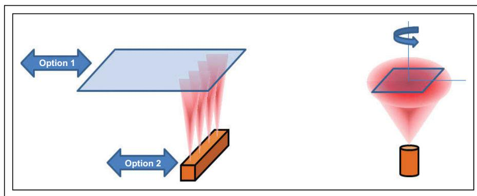
**Fig. 1:** At left, a simplified linear-source deposition process is depicted and at right, a point-source evaporation process. For the linear-source deposition concept, either the substrate (option 1) or the source (option 2) can be moved.
