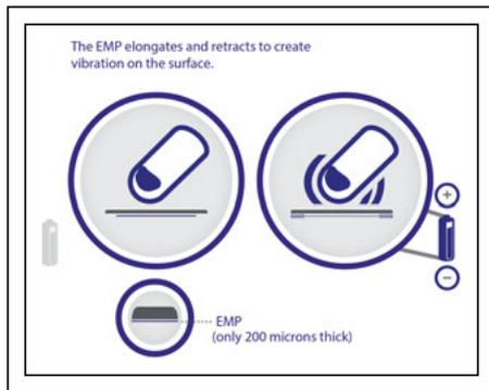
Fig. 5: In the image above, the electro-mechanical polymer is attached to the touch surface.
