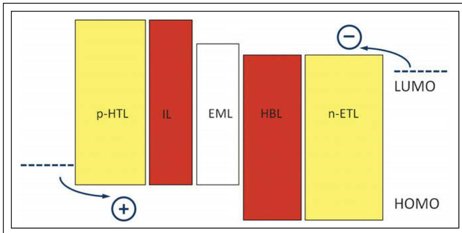
**Fig. 4:** An energy-level diagram of a typical OLED device depicts the highest occupied molecular orbitals (HOMO) and lowest unoccupied molecular orbitals (LUMO) of the organic materials used in the layer sequence.
