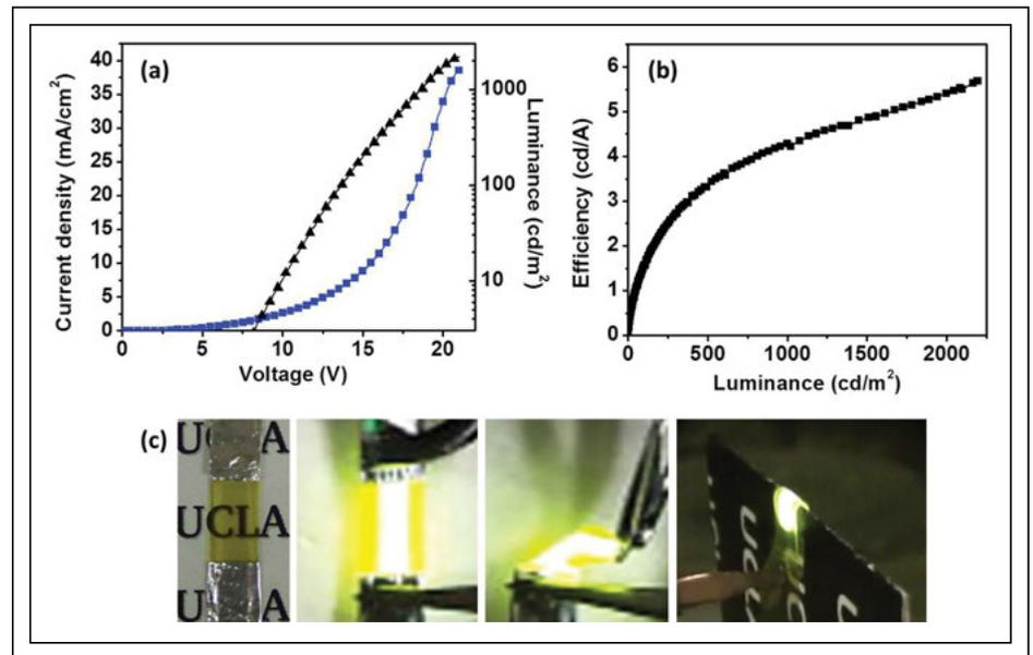
**Fig. 4:** At upper left (a) are shown the current-density–luminance–driving-voltage characteristics of an elastomeric PLEC device. (b) depicts the luminous-efficacy characteristics of the device. At lower left (c) are photographs of the PLEC (original emission area: 3.0 mm  $\times$  7.0 mm) unbiased, biased at 12 V, deformed to show light emission from both surfaces and folded around a piece of cardboard 400  $\mu$ m thick.
