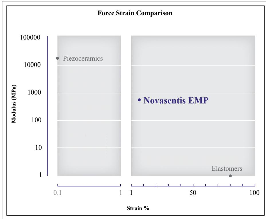
Fig. 3: The strain and modulus of PZT, dEAP, and EMP materials are compared.
